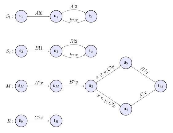
Figure 1: The synchronous transition diagram  $S_1 ||S_2||M||R$ .
